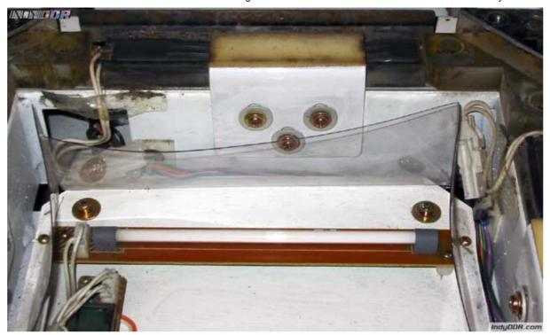
You can remove the sensors by sliding them out on the side where the wire comes out. Be careful not to bend the sensor too much as you do not want to bend or break anything inside it. I've found that this can be done either with or without removing the bracket above it first.
