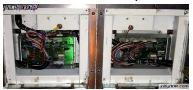
There's some wiring underneath the center panel on each side of the stage and there's a circuit board underneath the plate to the right of the up arrow on the Player 1 side of the stage and to the left of the up arrow on the Player 2 side of the stage. There's nothing else of much interest under the remaining plates.
